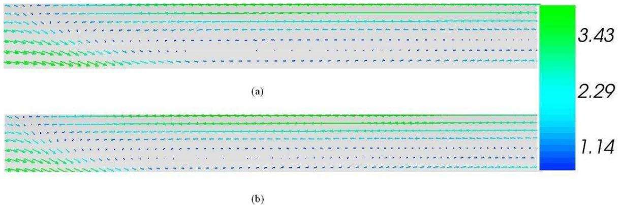
Figure 3: predicted velocities within the back-layering of (a) Case II (rough wall) and (b) Case I (smooth wall) at 900 s. Unit: m/s
