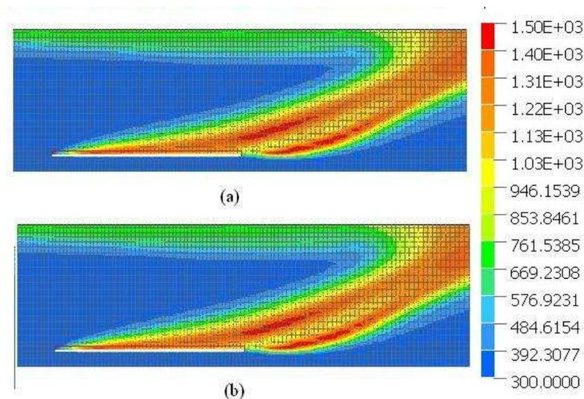
Figure 1: predicted temperature distributions by (a) the first mesh and (b) the second mesh. Unit: K
