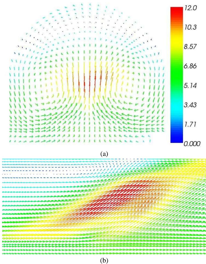
Figure 6: predicted velocity vectors in Case I. (a): cross section 12 m downstream from the fire, (b) central longitudinal plane. Unit: m/s
