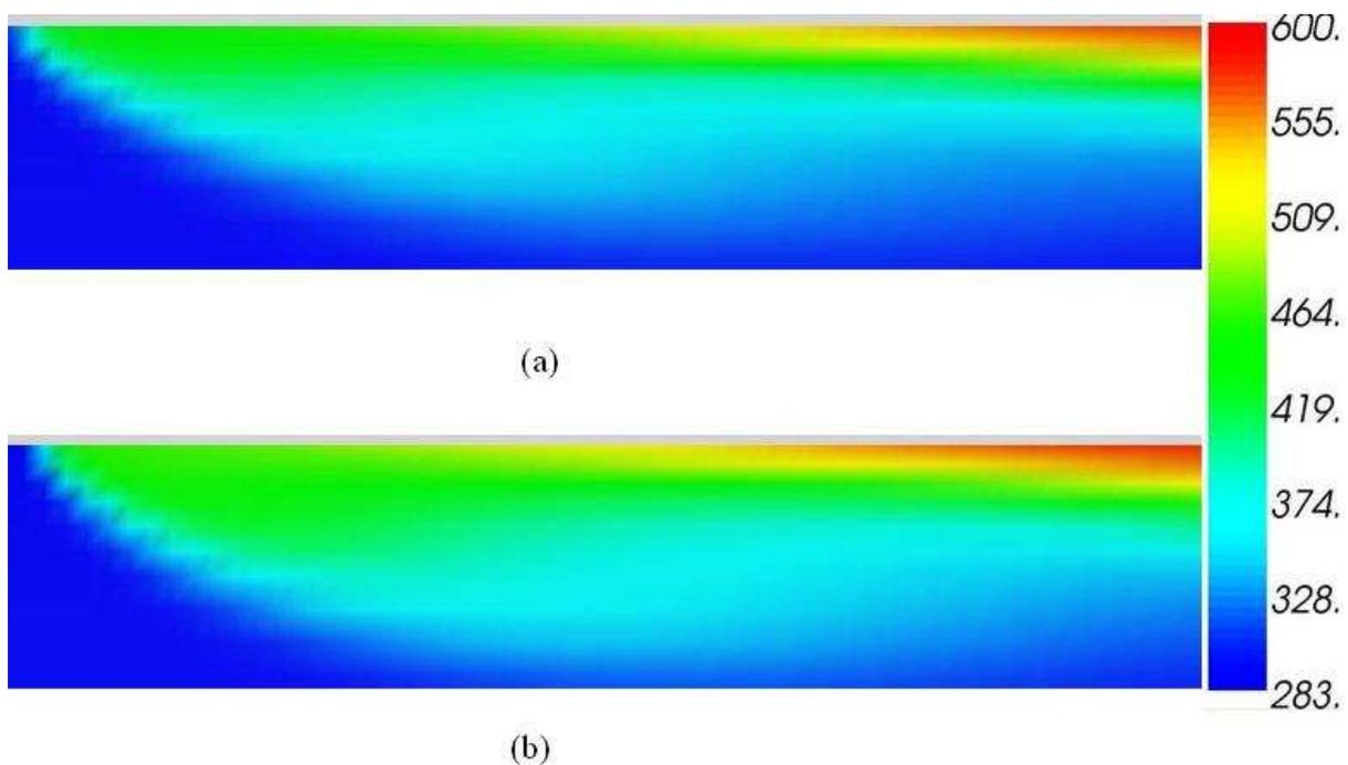
Figure 4: predicted temperatures within the back-layering (a) Case II (rough wall) (b) Case I (smooth wall) at 900 s. Unit: K
