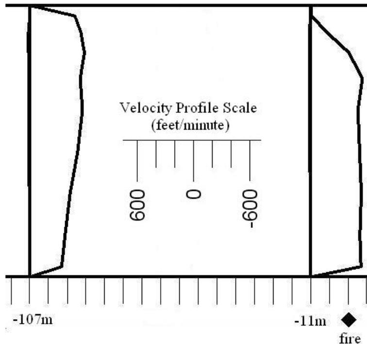
Figure 8: measured velocity profiles at -107m and -11m upstream from the fire at 969 s. (duplicated from <sup>2</sup>)
