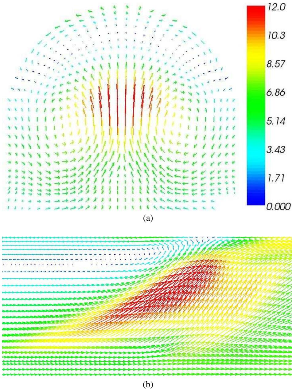
Figure 5: predicted velocity vectors in Case VI. (a): cross section 12 m downstream from the fire, (b) central longitudinal plane. Unit: m/s
