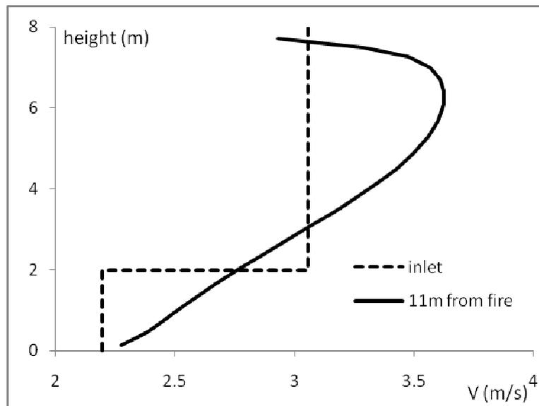
Figure 7: velocity profiles in Case III at inlet (-107 m) and -11 m from the fire.
